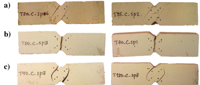
Fig. 7 – Typical failure modes of specimens tested at: a) 20 °C and 35 °C; b) 50 °C and 70 °C; and c) 90 °C, 120 °C.
